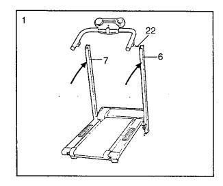
With the help of a second person, carefully tip the treadmill onto its right side. Hold the Base (80) against the Left Upright (7) and the Right Upright (not shown). Make sure the Base Pads (19) are on the bottom.
